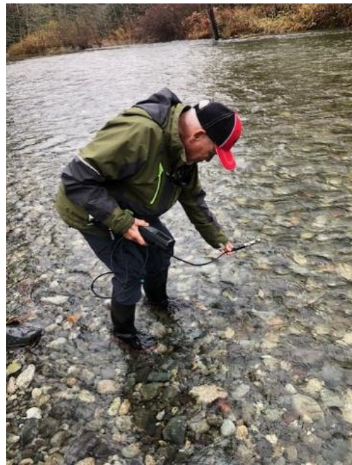
Photo 7: A volunteer taking a dissolved oxygen reading with a YSI meter at Nixon Creek
