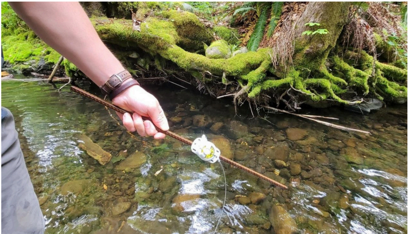
Photo 6. Bluetooth-enabled HOBO® MX Tidbit® 400 temperature logger secured to a piece of rebar prior to placement in Mayo Creek.
