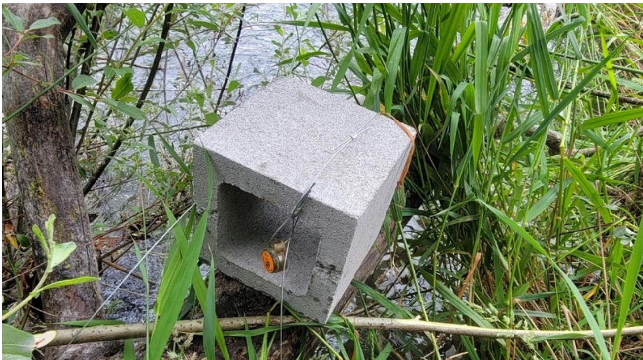
Photo 3. A HOBO® TidbiT® v2 temperature logger cabled to a cinderblock before placed in the Cowichan River above Fairservice Creek.
