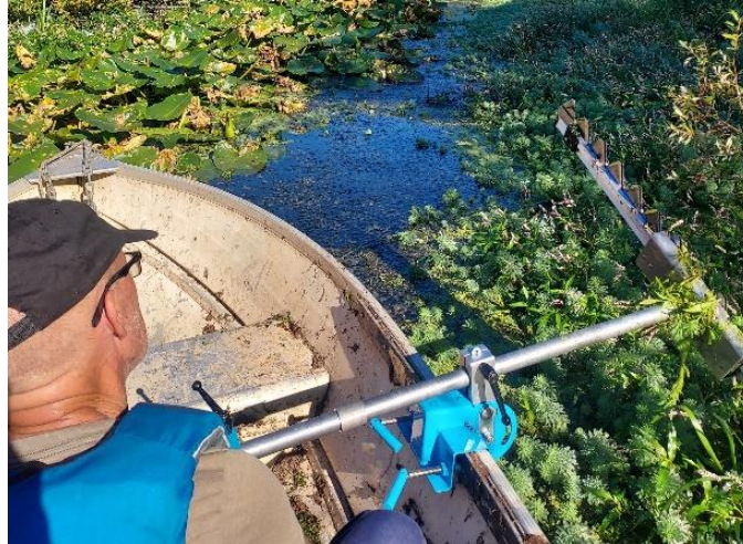
Figure 2: The aquatic weed mower attached to the gunwale of the boat.
