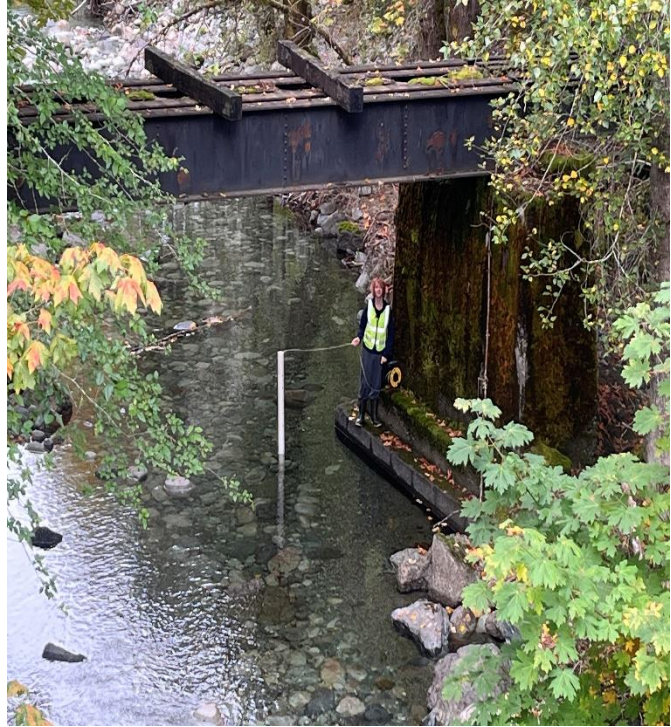
Aivars Liepa-Spence uses Dipper sensor to record water table levels in standpipes.
