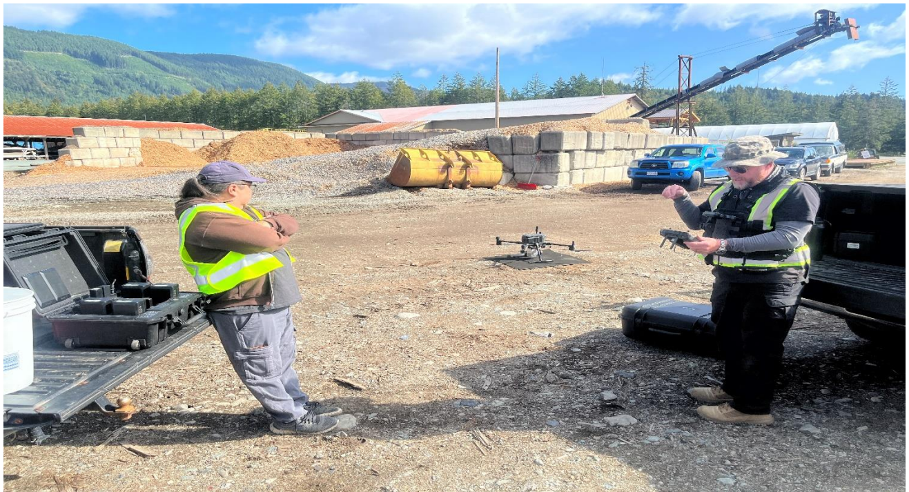
Ernest Pilfold (left) and Joe Henderson from Agile Drone conduct LIDAR data acquisition Oct. 2 nd 2024. This data will be used by Surveyor and Cartographer to map Meade Creek water table elevations.
