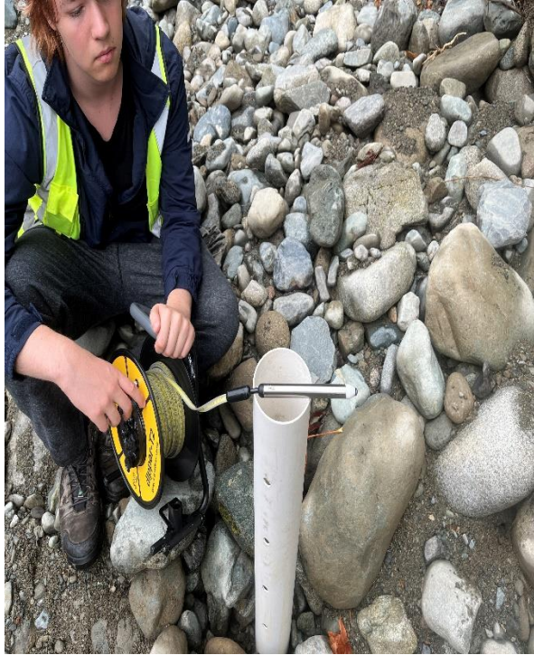
Aivars Liepa-Spence uses Dipper sensor to record water table levels in standpipes.
