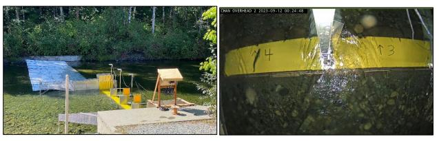
Figure 3: Traditional two-passage counting fence design used since 2019 (top) compared to the new low-flow design with four open passageways and overhead camera views (bottom).
