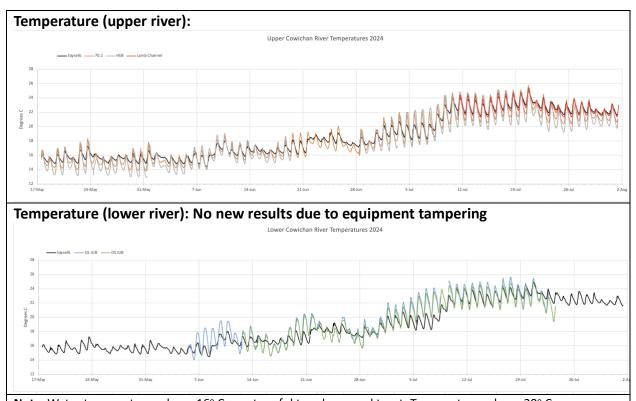
**Note:** Water temperatures above  $16^{\circ}$  C are stressful to salmon and trout. Temperatures above  $20^{\circ}$  C are extremely stressful and temperatures approaching  $24^{\circ}$  C can be lethal. Note: Data from Saysell's site from upper river added for comparison.
