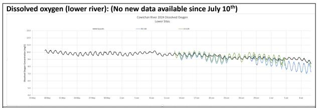
**Note:** Diurnal DO fluctuations result from algal respiration. The Saysell Site is located in the upper river above the sewage outfall and represents preferred range in DO diurnal fluctuations. Wide diurnal fluctuations indicate excessive algal growth which can be stressful and in extreme cases lethal to fish populations.
