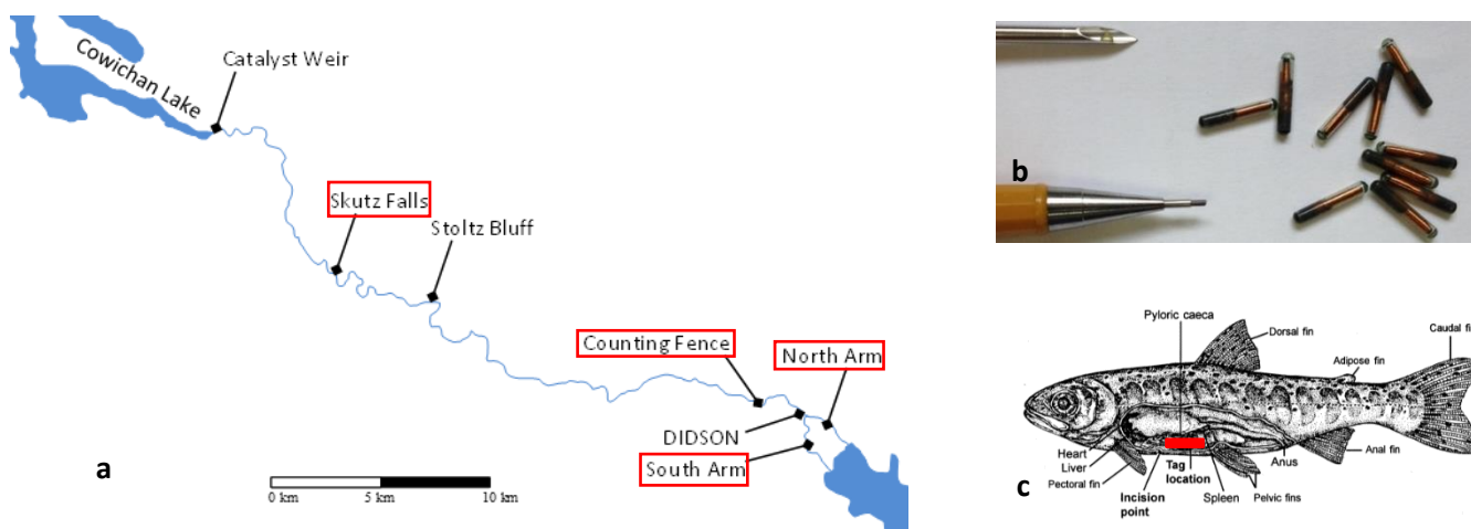
Figure 10: (a) Locations of PIT antennas (red) along with other places of interest in the Cowichan River. (b) PIT tags and implantation needle compared to the size of a mechanical pencil. (c) Anatomy of a salmon smolt with tag location in red.
