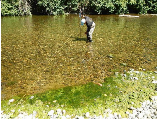
Photo 3. Cross-stream view of North Arm flow site, 40 m downstream of bifurcation, Jul 31, 2015. Q=3.619 \text{ m}^3/\text{s} .
