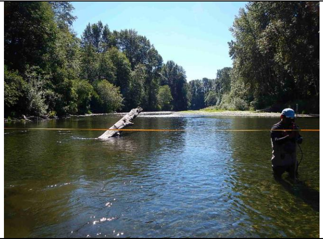
Photo 2. Downstream view of "Mainstem above Bifurcation" flow site, Jul 31, 2015. Q=3.619 \text{ m}^3/\text{s}
