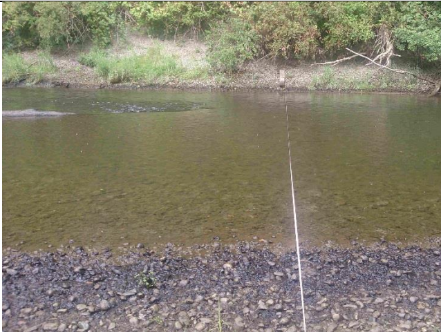
Photo 5. Cross-stream view of South Arm flow site just above Hatchery Channel, Aug 10, 2015. Q=1.664 \text{ m}^3/\text{s}
