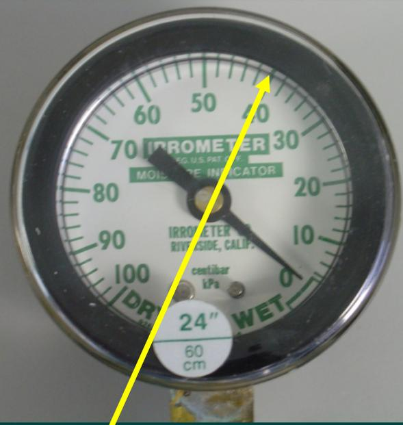
**An irrigation system in a sandy loam soil with a root depth of 1 m. Is scheduled to begin irrigation when the available water has been depleted by 50% Irrigation should start when the sensor Reaches 40 centibars**
